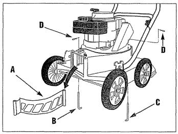
Figure 8: Shredder screen removal.
